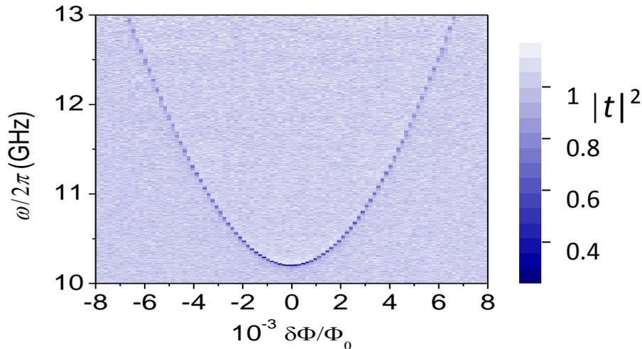
Spectroscopy of the artificial atom. Power transmission coefficient  $|t|^2$  versus flux bias  $\delta\Phi$  and incident microwave frequency  $\omega/2\pi$ .
