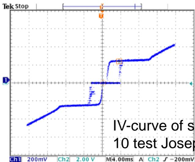
The chips were fabricated using standard IPHT Nb process with 1 kA/cm<sup>2</sup> critical current of JJs
