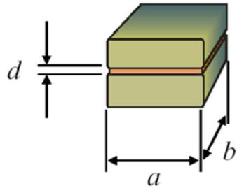
tunnel barrier thickness  $d$
